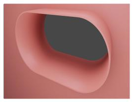
Make sure the conduit opening is clean from dirt, rust, oil and welding spots.
