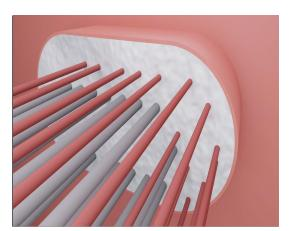
The space of 20mm must be filled with the IBMO pyro Putty. Make sure the surface is smooth. To create this use a water-and soap mixture. Use a wet sprayed hand to push the putty into gaps, small spaces between cables and to smoothen the surface. Now you have created a fire-, gas- and watertight penetration.
