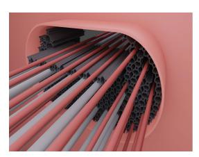
Fill the penetration with IBMO starclover profiles. Use the single profile or the multi strips profiles to fill. Leave 20mm space on each side of the coming.
