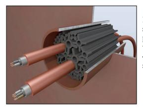
Fill the penetration with IBMO star/clover profiles. The length of the profiles depends on the length of the welded in conduit sleeve minus 40mm. Leave 20mm space on each side of the coming.
