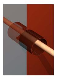
Pipe or cables can be installed through welded in pipe sleeve.
